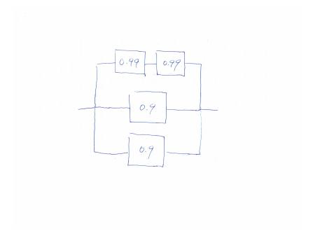
Assume that the probability that a device is functional does not depend on whether or not other devices are functional. What is the probability that the circuit operates?
